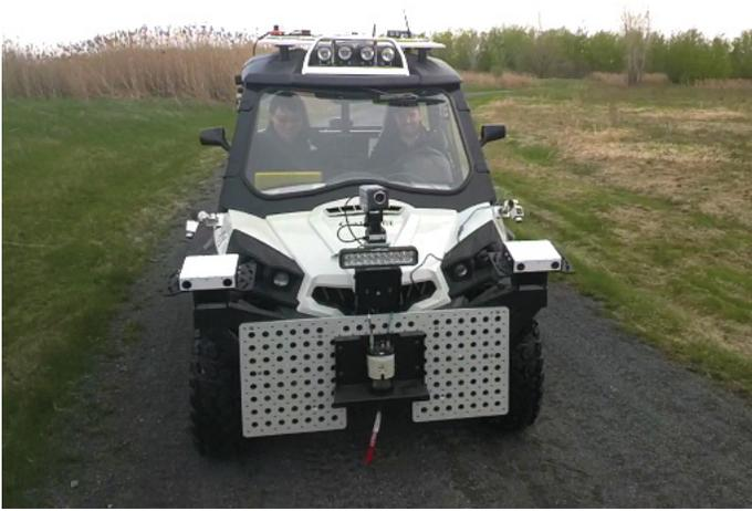
Figure 3–11: The participant, sitting in the SL-Commander’s passenger seat, collaborated with our adaptive boundary tracking agent during the APEX interactive driving field demonstrations. A human driver was also present and provided redundant safety duties by maintaining access to the vehicle’s brake pedal and emergency stop buttons.
